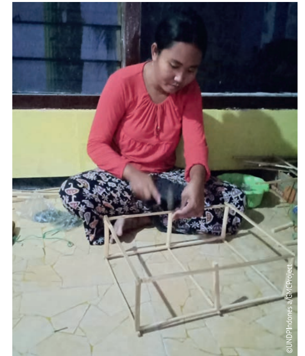
Figure 6. A woman in Pamekasan repairs bamboo traps using bamboo that has been cut into small pieces and sanded.
